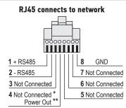
4 Cond. 26AWG modular cable with RJ9 on one end and RJ45 other end - (RTS, Z-Wave®, ZigBee modules)
